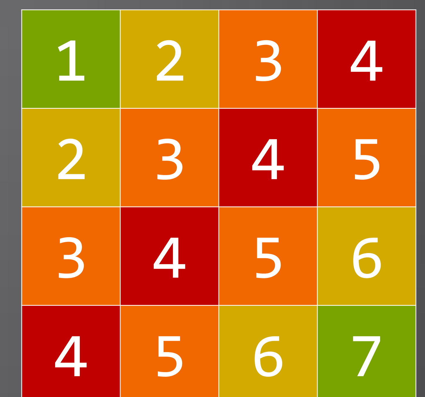
Figure 5: Hot Zones Darker, or "hotter" cells represent regions in the matrix which have a higher potential for parallelization, because these regions are independent of each other.
